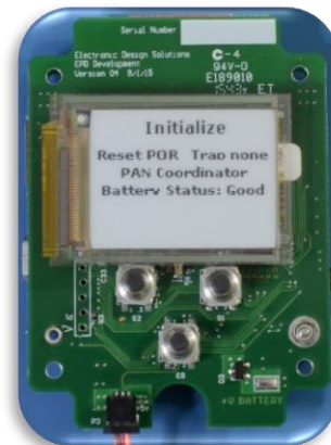
Figure 9. Reset, Trap and Battery status
