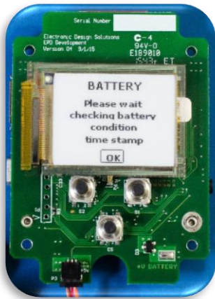
Figure 17. Initializing Battery test
